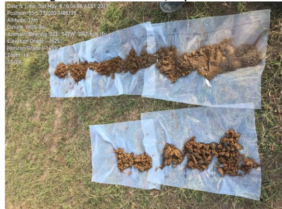
Figure 2: SS08 Soil Profile, Depth to 1.2 m
