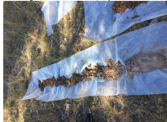
Figure 2: SS09 Soil Profile, Depth to 0.8 m
